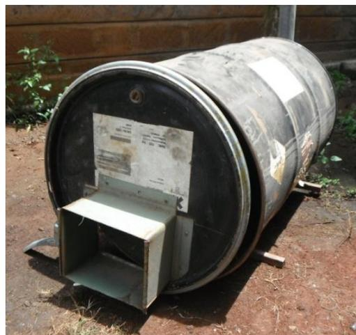
*Traditional earth kiln (M. Njenga) vs a drum kiln of about US\$50 with efficiency of 30% (N. Oduor)*
