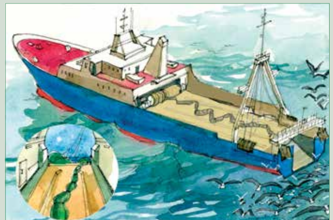
Figure 1. Net binding reduces the amount of time the net is on the surface.
